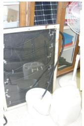
We have tested all three of the solar hot water heaters. It took us a while to actually start our testing because the water leaks. The water would leak out of where the hose would connect to the bucket and also where two hoses connect to each other. After a lot of altering, we finally got them to stop leaking and got some data, our findings are in graph below.
