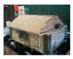
By looking at the graph above we can see that we need to target the ceiling, around the windows and inside the walls because they lose the most heat. We realized that the ceiling needed extra insulation because it was the steepest point and all of the hot air rose and the escaped from the roof.
