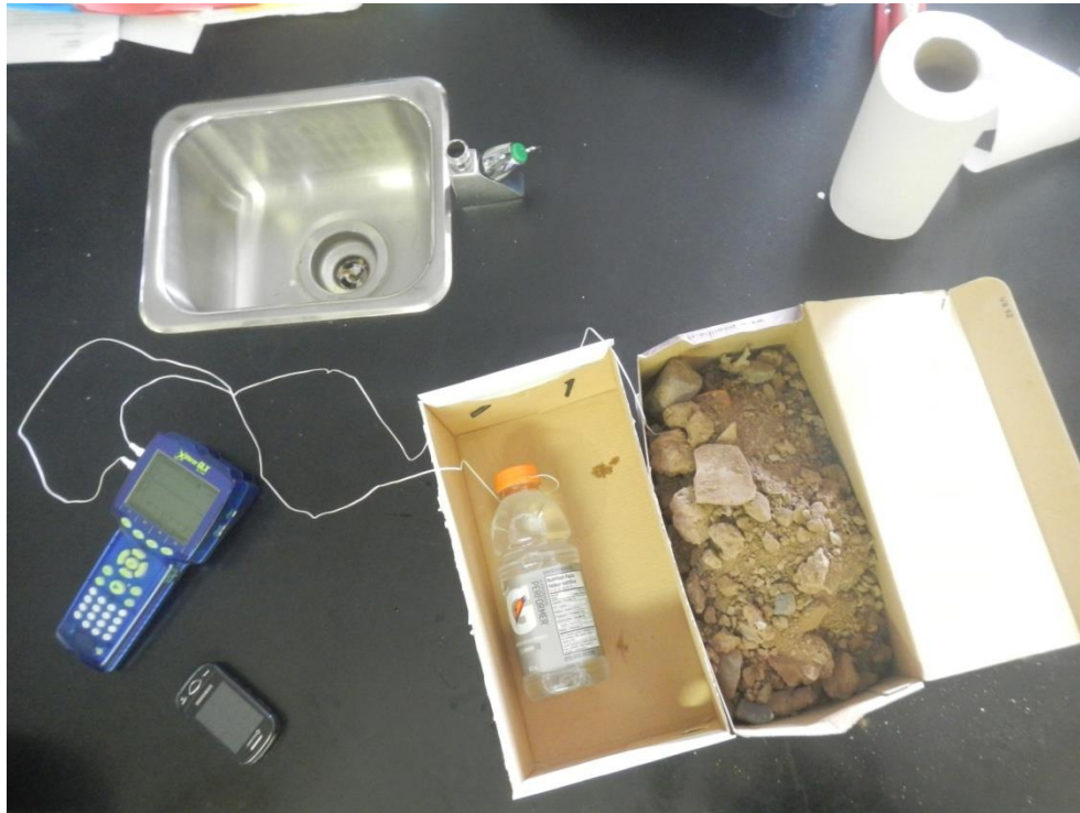
Figure 2.1: Testing which medium, air or dirt, serves as a better insulator
